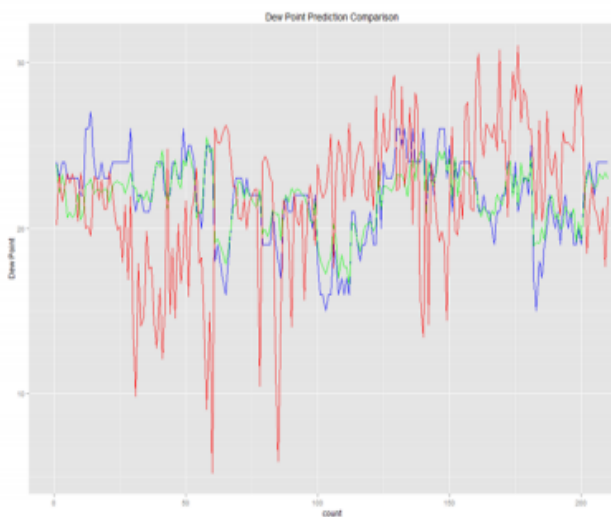
Fig. 6. Actual output, prediction by normal equation and prediction by gradient descent for dew-point
